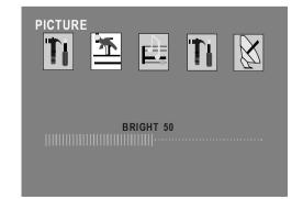
Press button 2: adjust brightness to lighter level. Press button 3: adjust brightness to darker level. Press button 1 to confirm setting. [Brightness adjustable level: 0-100 . Preset: 50]
